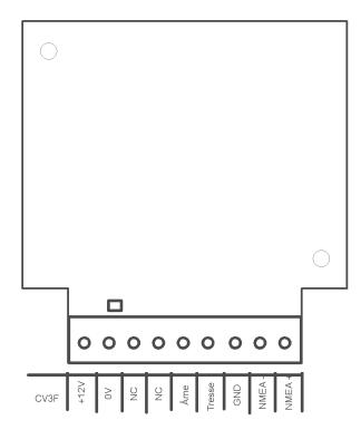
Use the supplied screwdriver to preserve the screw terminals. Connect the 12V power supply (9.5 to 14 VDC). Blue 0V / Brown + 12VDC.
