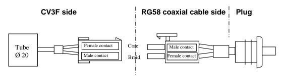
The plug at the end of the tube has a hole to allow the passage of coaxial cable RG58 and a small hole (1.5mm), sufficient to assure a natural weatherproofing and at the same time to stabilize the internal and external pressures on CV3F. During installation, care must be taken to ensure that this hole is not closed, and to be left in the same atmospheric pressure as the sensor itself.
